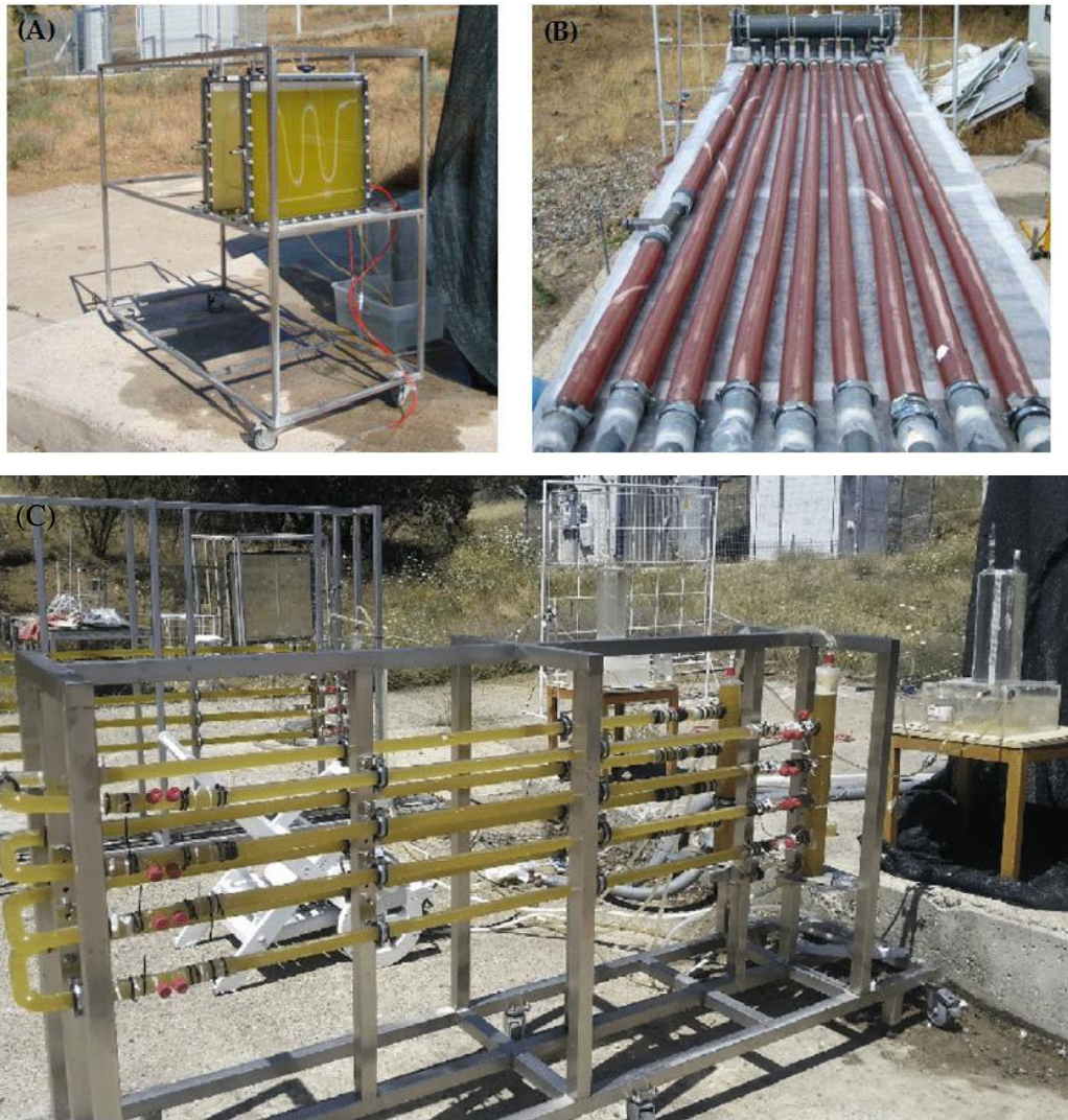
Figure 1.8.1 Panel reactors, continuous tubular reactors, and tubular reactors with u-bends as some of the previously experimented reactor types in the METU Hydrogen Research Laboratory (Androga et al. , 2012, Kayahan et al. , 2016)
