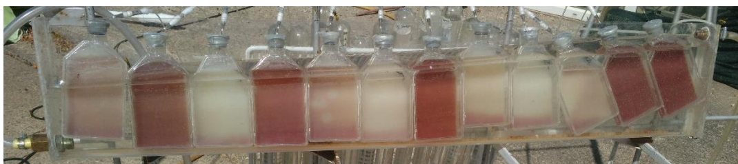
Figure 2.3.2 300 mL panel plexiglass reactors inside the water bath during the outdoor experimentation.
