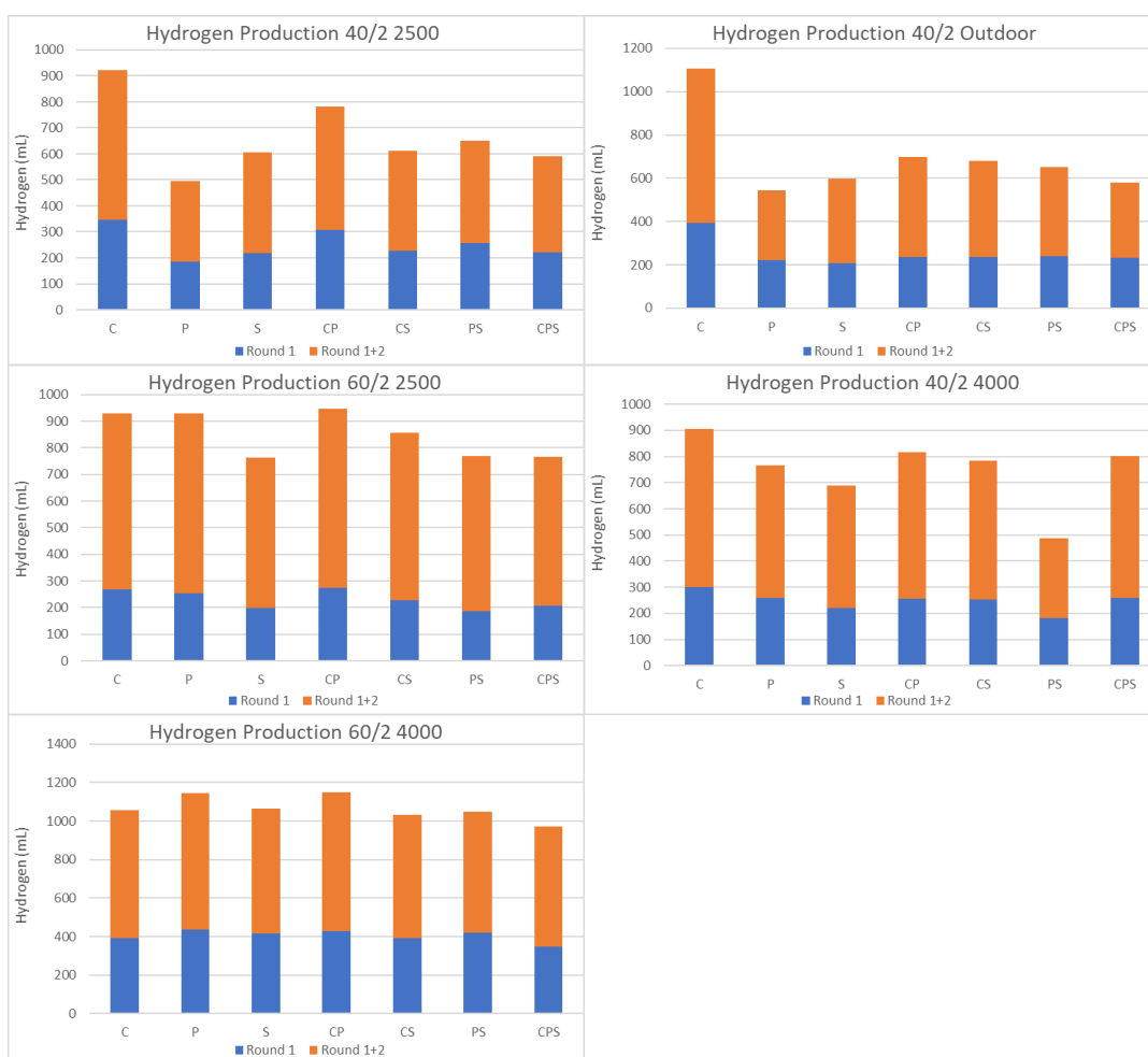
Figure 3.4.22 Total H 2 Production in round 1 and round 1 + round 2 for 150 mL single cultures and double and triple co-cultures of R. capsulatus hup- (YO3), Rp. palustris (DSMZ 127) and R. sphaeroides O.U.001 (DSMZ 5864) in an immobilized setting, cultivated on BP medium supplemented with 40 mM Acetate/2 mM Glutamate and 60 mM Acetate/2 mM Glutamate at 30 °C under deoxygenated atmosphere and uninterrupted illumination of 2500 lux and 4000 lux for indoor, and under sunlight for outdoor.
