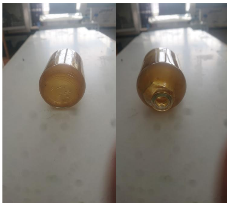
Figure 2.3.3 150 mL glass reactors covered internally with agar-bacteria matrix of 2 mm thickness.
